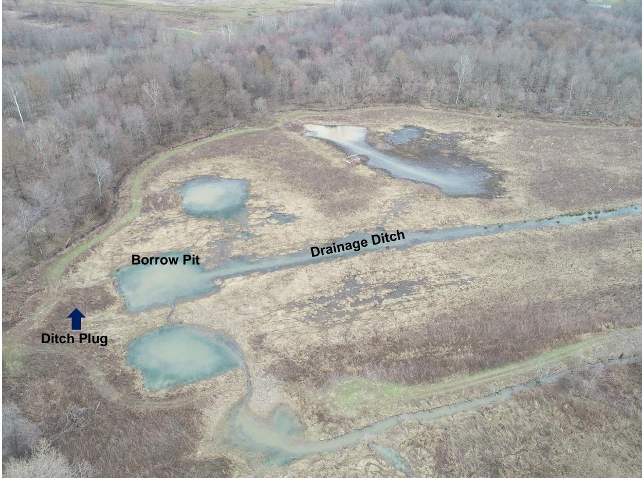
**Figure 1.7** Drone imagery shows the ditch plug and borrow pit method used to hydrologically restore the wetland on HOPK. This restoration method kept approximately 56% of the easement's surface area inundated when water levels were at an average depth.
