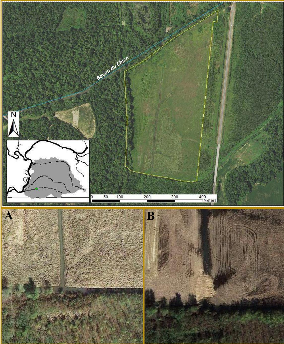
**Figure 1.1** A drainage ditch plug is one of the hydrological restoration tools used by USDA-NRCS on WRP easements. Satellite images of HWST shows the drainage ditch before (A) and after (B) the ditch plug was installed.
